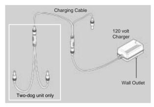
The battery charger and charging cables allow you to charge both the transmitter and receiver at the same time. The battery charger is designed for a 120-volt wall outlet. (European 230-volt AC chargers and 12-volt field charger for Lithium-Polymer batteries for your automobile are also available.)
