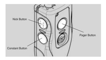
The transmitter for the **dogtra** Element 300M single dog unit has three buttons (one on the face of the transmitter, two on the left side).
