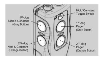
The **dogtra** Element 302M two-dog unit has four buttons and a toggle switch on the transmitter. (Two on the face of the transmitter, two on the left side)
