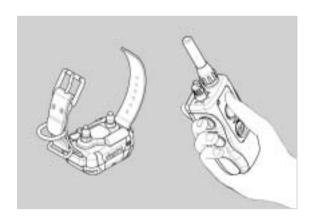
1. To activate your **dogtra** Element 300M Series place the red dot on the back of the transmitter to the red dot on the collar/receiver. Hold the two red dots together for a moment until the green colored LED indicator light comes on. The indicator light will blink every two seconds showing the unit is charged and ready to use. (If the indicator light emits a red color, the batteries need to be charged.)
