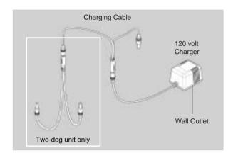
The battery charger and charging cables allow you to charge both the transmitter and receiver at the same time. The battery charger is designed for a 120-volt wall outlet. (European 230-volt AC chargers and 12-volt car chargers are also available.)
