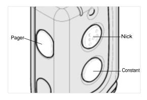
The transmitter for the *dogtrd* 200NCP GOLD SERIES has three buttons (two on the face of the transmitter and one on the side).
