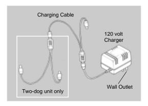
The battery charger and charging cables allow you to charge both the transmitter and receiver at the same time. The battery charger is designed for a 120-volt wall outlet. (European 230-volt AC chargers and 12-volt field charger for your automobile are also available.)
