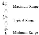
If your finger touches the antenna near the dial on the top of the transmitter, the actual range may be reduced.
