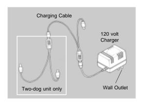
The battery charger and charging cables allow you to charge both the transmitter and receiver at the same time. The battery charger is designed for a 120-volt wall outlet. (European 230-volt AC chargers and 12-volt field charger for your automobile are also available.)
