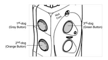
The transmitter for the *dogtrà* 1803NC has three buttons; The Gray (1st dog) button corresponds to the receiver with the black collar strap. The Orange (2nd dog) button corresponds to the receiver with the orange collar strap. The Green (3rd dog) button corresponds to the receiver with the green collar strap.
