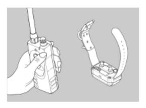
1. Turn the collar on by pressing the button on the back side of the collar receiver. The indicator light will come on for a moment then blink once every two seconds, showing that the collar is ready to use. (If the indicator light is red, the batteries need to be charged.) Place the test light on the contact points of receiver and hold it there.
