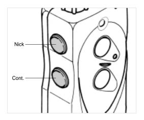
The transmitter for **dogtrd** 1800NC has two buttons. The top is the Nick button and the bottom is the Constant button.
