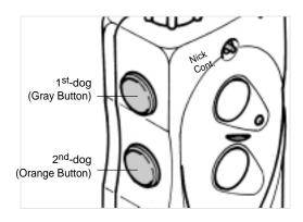
The transmitter for the *dogtrd* 1802NC has two buttons; The 1802NC has two buttons on the side of the transmitter. The gray button corresponds to the receiver with the black collar strap and the orange button corresponds to the receiver with the orange collar strap. The toggle switch at the top of the transmitter allows you to choose between Nick and Constant type of stimulation.
