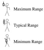
If your finger touches the antenna near the dial on the top of the transmitter, the actual range may be reduced. Additional environmental factors may also affect the range of your unit.
