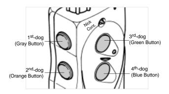
The transmitter for the *dogtrd* 1804NC has four buttons; The Gray (1st dog) button corresponds to the receiver with the black collar strap. The Orange (2nd dog) button corresponds to the receiver with the orange collar strap. The Green (3rd dog) button corresponds to the receiver with the green collar strap. The Blue (4th dog) button corresponds to the receiver with the blue collar strap.
